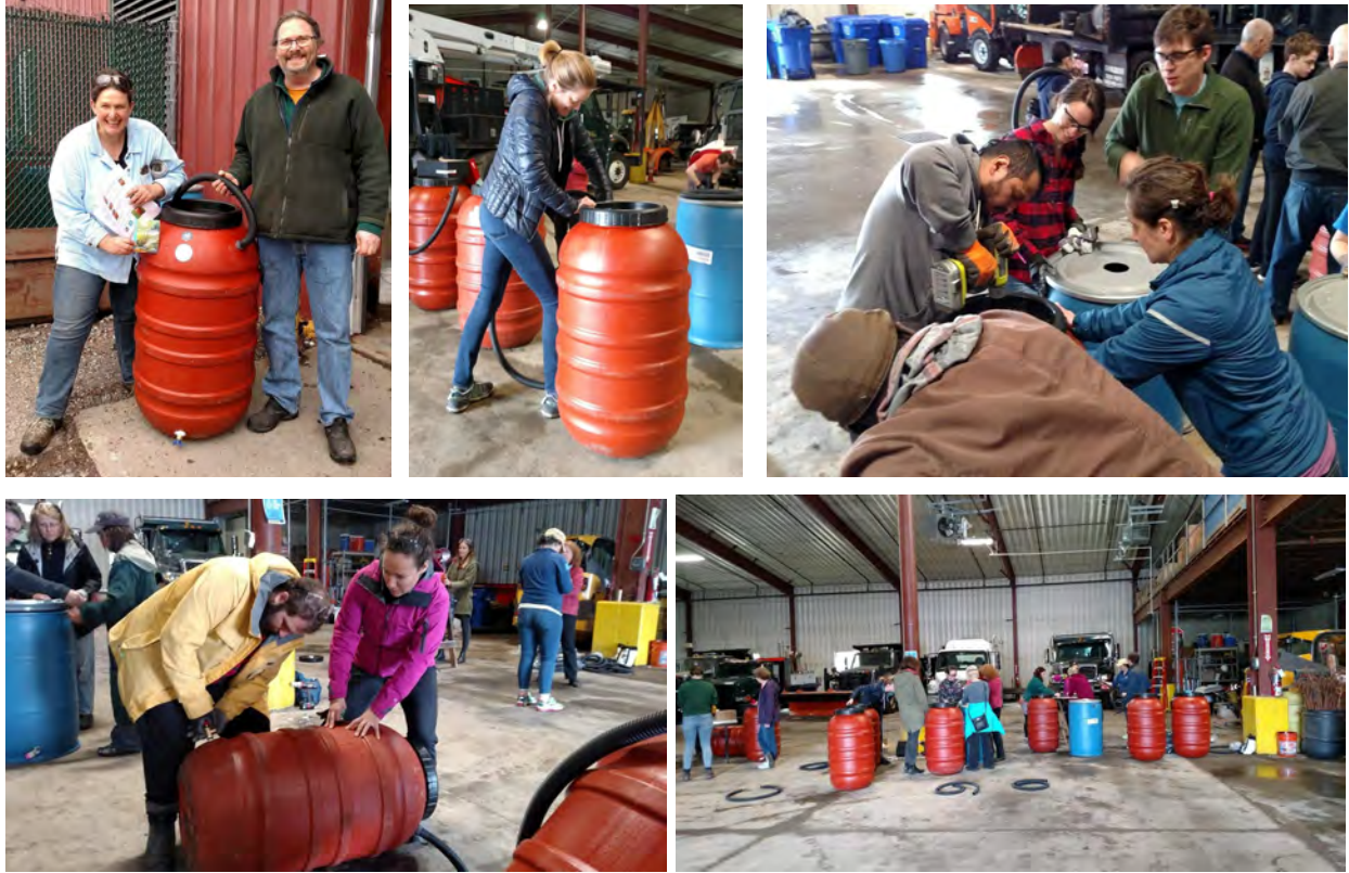
Figure 3: Participants at the Burlington Rain Barrel Workshop drill, assemble and caulk their new barrels.
